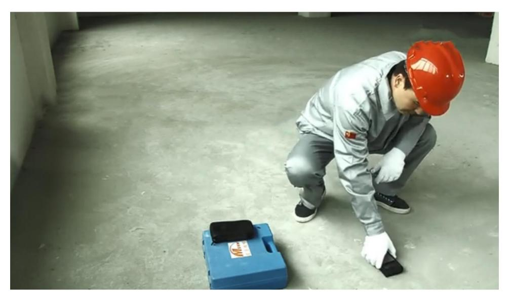
Using the CCM moisture tester to detect the ground of water ratio, the test result should not be more than 4%.
