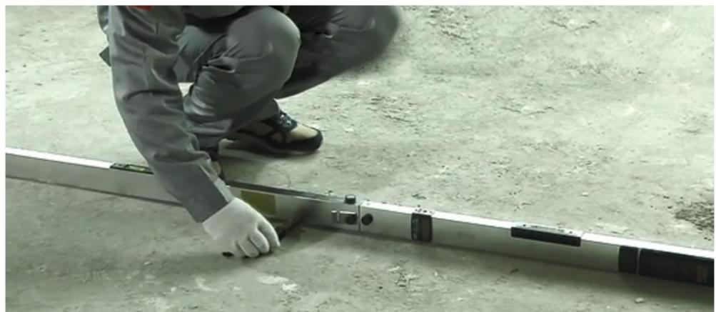
The detection result of surface flatness tester that the height difference within a two-meter straight line shall be less than 5mm. (Both ends of the flatness detector shall be fitted with the ground).
