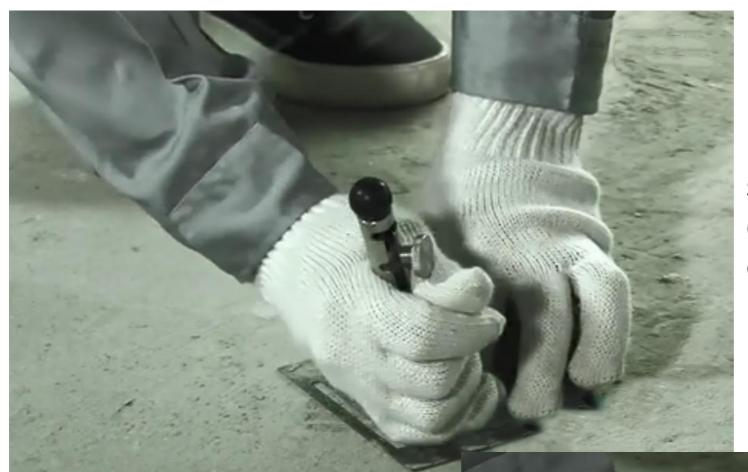
Using the hardness scratching tester to detect the hardness of ground surface.
